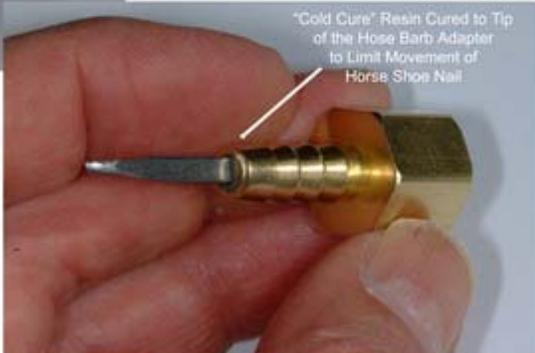
Now assemble by screwing the hose barb adapter to one end of the pipe, insert the wood dowel and tighten the pipe cap to the other end. Note the good "front to back" stability. If the nail should loosen while in use just tighten the pipe cap.
