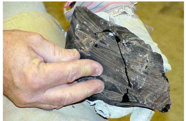
Here is the same flake removed from the rock. Note that it is a portion of that same spall cone we looked at in the beginning when a BB hits plate glass. Doc will simply remove more portions of similar cones at places (and sizes) of his choosing, until he ends up with the desired results.
