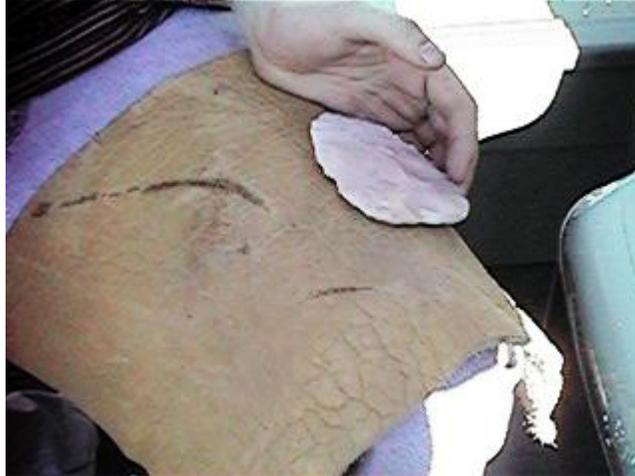
*The picture above shows how easily the angle can be determined on the knee. The hand would then rest flat on the preform to press it into the pad and prepare it for the strike.*
