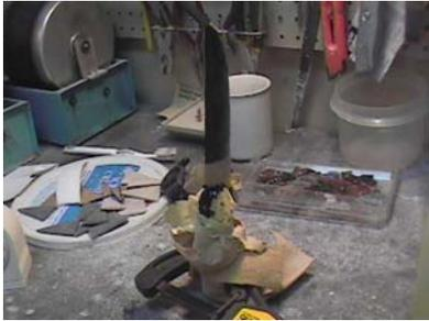
black and when it dries it will look very similar to pine pitch. Set a timer for 15 minutes and fill in the slot completely with the glue. Now we do a little clean up making sure none of the glue runs and let it sit for 10 minutes. If you made the mistake like I did and the blade does not sit still then you will have to watch it moving it back into place.
