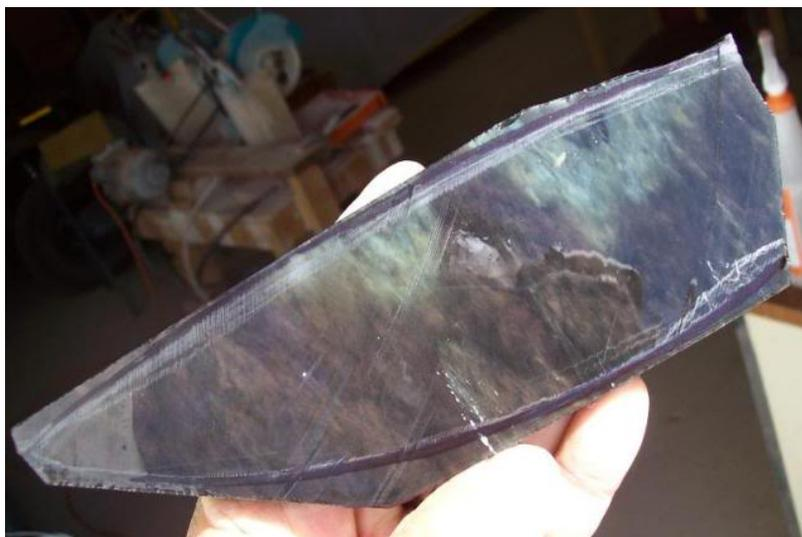
Take a slab, orient it the way you want, mark out the shape and trim with a tile saw. Closer trimming here save diamonds later! I slab my own with an 18" Highland Park.
