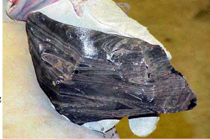
Note the heavy leather glove on his left hand, and the thick leather pad on his leg. The flakes he'll be removing are said to be the sharpest edge known to man. Because of the conchoidal breakage characteristics of obsidian, the edge produced is feathered out to an edge one molecule thick, far sharper than the best surgical steel.
