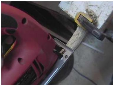
Now take your saw and cut each line from start to mark. Then go down the center and angle it to each side to remove all the middle antler. You can now cut off the remaining pieces with a hand saw. You can finally clean it out with a file making sure not to remove too much from the sides. Test your blade into the slot to make sure it fits and nothing more needs to be removed.
