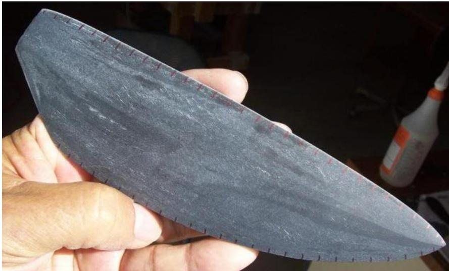
Grind out the shape then grind both faces into a convex shape. Leaving a median ridge down the middle helps the flakes terminate smoothly. I'm not always successful. Rough it out with the coarse wheel leaving about a 1/16" flat on the edge so you don't rip the edge off. Smooth it out removing all the grind scars with the fine wheel. Start with thicker slabs to allow for grinding removal.
