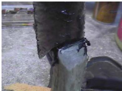
Ding Ding! The timer goes off. Immediately set it again for another 15 minutes. The glue should be like play dough now. Remove the tape. Now clean up the glue with a flattened nail or similar. What you are doing here is making sure there are no lumps, no glue
