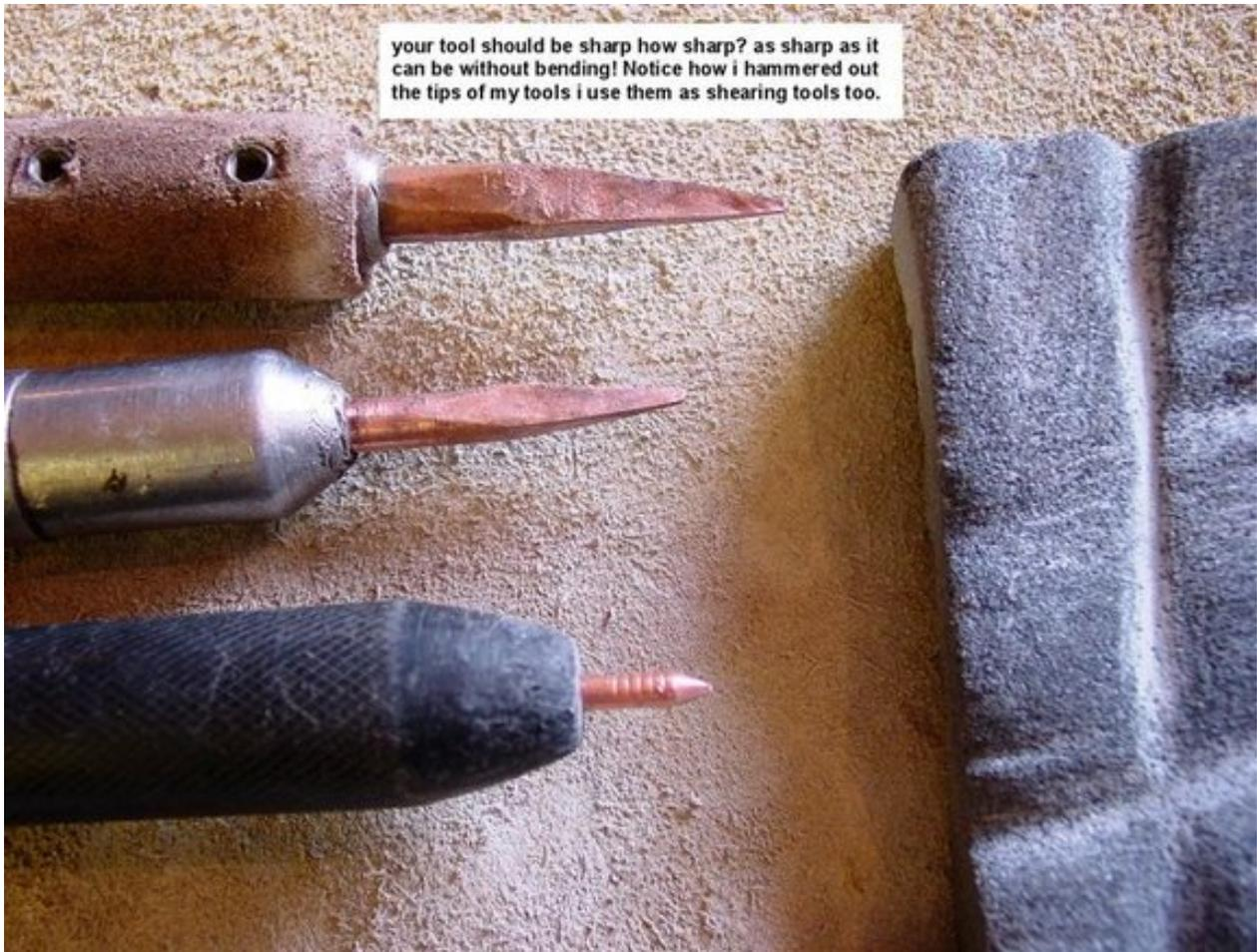
your tool should be sharp how sharp? as sharp as it can be without bending! Notice how i hammered out the tips of my tools i use them as shearing tools too.
