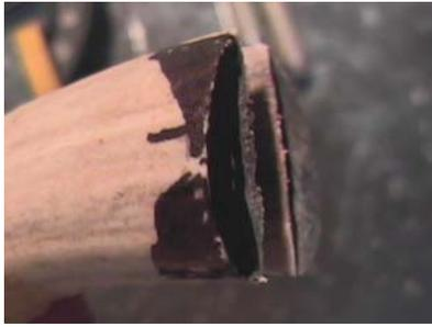
Now as an optional method we can round the sides of the antler. Take your marker and mark the areas to be removed. Now take it to the grinder and remove these areas as well as cleaning up anything on the base of the antler. If you have no grinder then this can be done with steel rasps and 60 grit sand paper. I did the hand method for years and it can be done but takes a lot longer. Finally, once in shape, take 120 grit then 220 grit sand paper and sand it down smooth.
