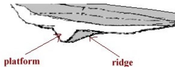
*Another example of a platform set up on a ridge. The platform has to be at an angle less than 90 degrees. The relative dimensions of the platform, ridge, and preform in this drawing have been exaggerated for clarity. As the preform gets thinner the platforms get smaller too. Everything gets more subtle as you near the final form.*
