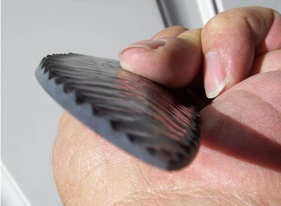
Back to the grinder (fine wheel) and bevel the working edge back the other way to flake the other face. Repeat above, placing the tip of flaker in the middle (the strongest part) of each delta. No measuring or marking needed as the deltas should be spaced just right.
