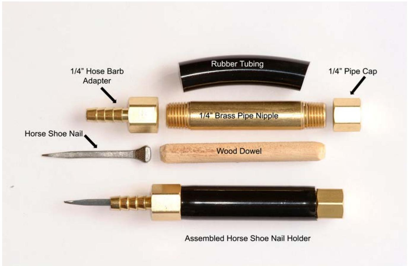
Fill the inside of a hose barb adapter about half way up with resin and insert a lubricated horse shoe nail. Allow to set and tap out the nail. Nails of similar type are now interchangeable and have good "side to side" stability.
