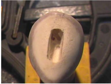
Now we have two choices. One choice is to use a drill with various sizes of bits and drill out several holes to the depth of the tang. You can clean up the hole marks with knives and files. The hole will look like this. Then the knife will fit in the hole. Epoxy or pine pitch will hold it into place.
